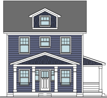
Front Elevation - Reverse Gabled Roof
