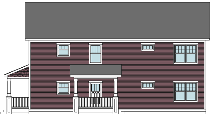
Left Side Elevation - Gabled Roof
