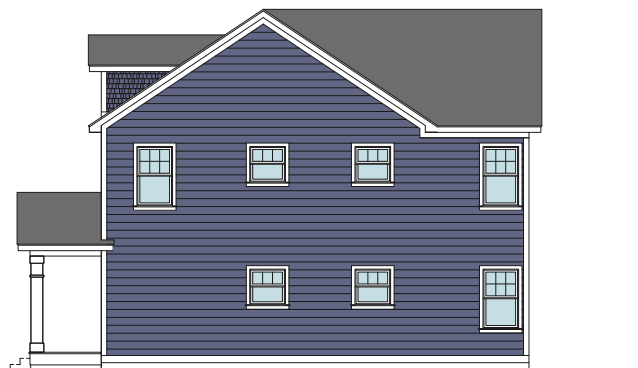
Side Elevation - Reverse Gabled Roof
