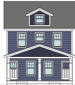
Front Elevation - Reverse Gabled Roof
