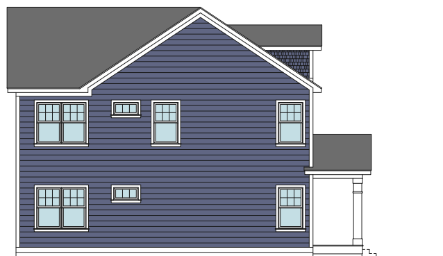
Side Elevation - Reverse Gabled Roof
