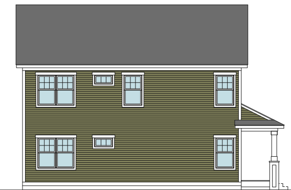
Side Elevation - Gabled Roof
