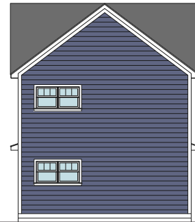
Back Elevation - Reverse Gabled Roof
